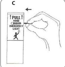
Insert the RED TAMPER EVIDENT PIN into the side of the dispenser and continue to push the pin through all three holes until it stops (See Illustration C). The pin is self locking, and CANNOT BE REMOVED WHITHOUT BREAKING THE PIN.
